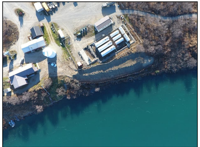
A drone pic of the sheet pile wall, protecting our bulk fuel farm. Courtesy of Karl Hill.
