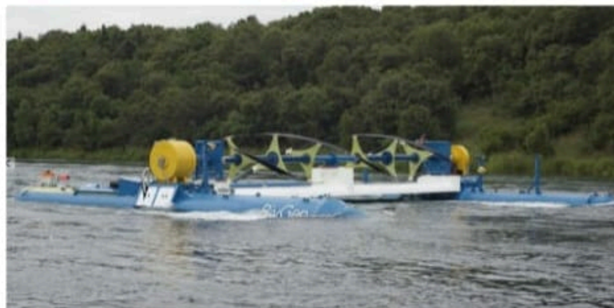
Figure 1. RivGen Power System in 2019 (prior to submerging)
